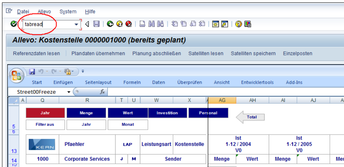
Figure 27.1: Entry of the TABREAD command to activate debugging
