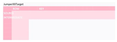
The aim of the jumper is to copy data from a source (usually the planning mask) into one or more rows of a structured target table (usually a satellite) by double-clicking. The number of rows to be appended to the table can either be fixed, specified by the user, or determined dynamically via an intermediate table.
